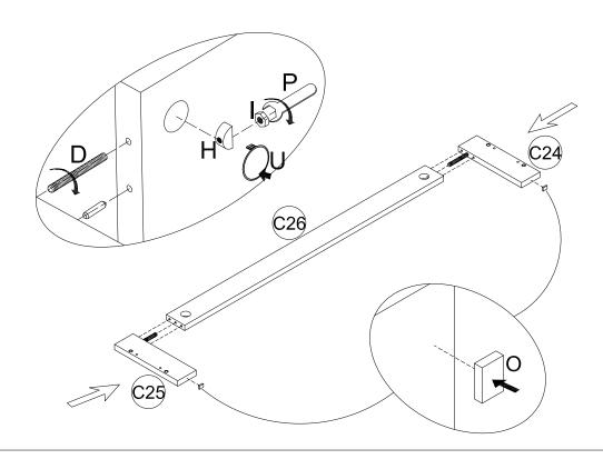
Step 26: Attach the Left Connect Panel(C24)and Right Connect Panel(C25) to the Left Side Panel(C20) and the Right Side Panel(C21). And use Wrench(P) to secure Half Round Nuts(H) and Hexaganal Nuts(I).
