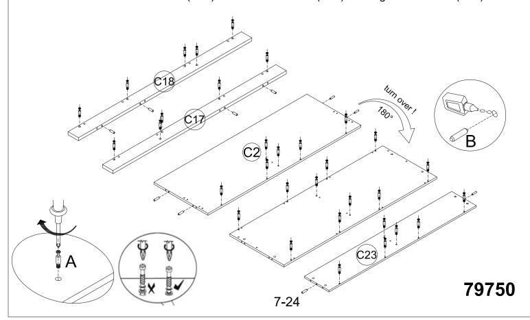
Step 4: Insert the Dowel(B) into the Headboard Left Side Panel(C3)and
