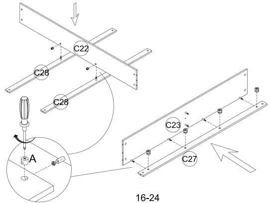
Step 21: Attach Footboard Panel(C23) to the Middle Support Panel(C22). And use a Phillips Head Screw to turn the Cam Lock(A) to lock into the head of the Cam Pin(A).
