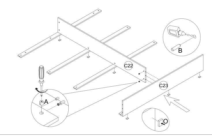
Step 22: Attach Right Side Panel(C21) to the Rail(C27/C28) and Footboard Panel(C23). And use a Phillips Head Screw to turn the Cam Lock(A) to lock into the head of the Cam Pin(A).
