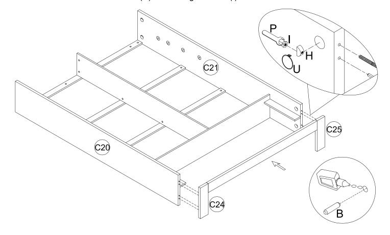
Step 27: Align the Dowels(B) in the Headboard to the Left Side Panel(C20) and the Right Side Panel(C21). Use Wrench(P) and Hey key(N)to secure Bolt(C) and Half Round Nuts(H) and Hexaganal Nuts(I).
