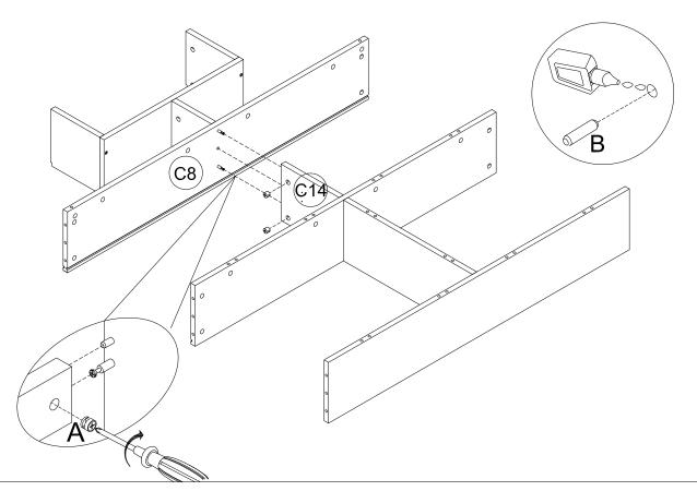
Step 9: Attach Headboard Right Side Panel(C4) to the Headboard Bottom Panel(C7) and Shelf Panel(C8/C9). And use a Phillips Head Screw to turn the Cam Lock(A) to lock into the head of the Cam Pin(A).
