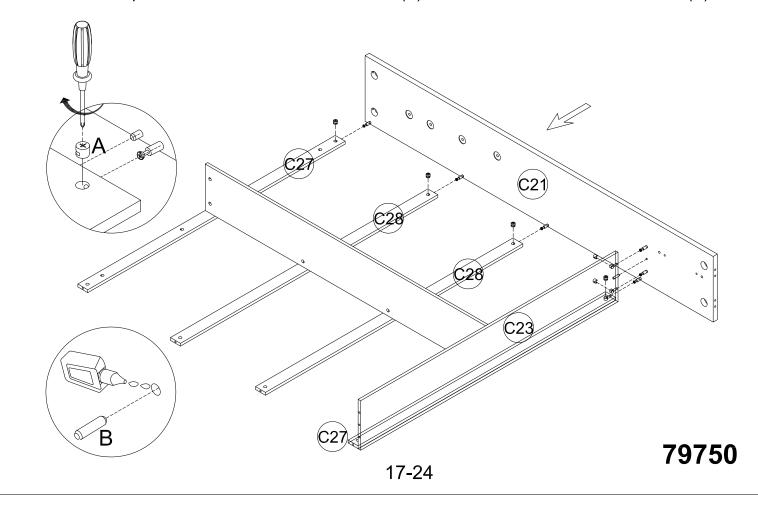
Step 23: Attach Left Side Panel(C20) to the Rail(C27/C28) and Footboard Panel(C23). And use a Phillips Head Screw to turn the Cam Lock(A) to lock into the head of the Cam Pin(A).
