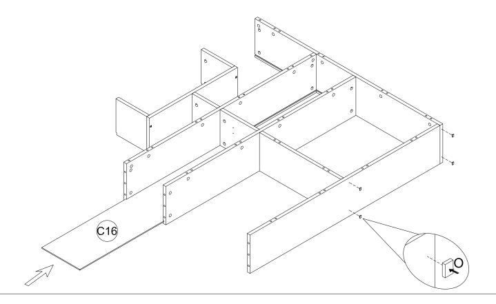
Step 11: Attach Headboard Left Side Panel(C3) to the Headboard Bottom Panel(C7) and Shelf Panel(C8/C9). And use a Phillips Head Screw to turn the Cam Lock(A) to lock into the head of the Cam Pin(A).
