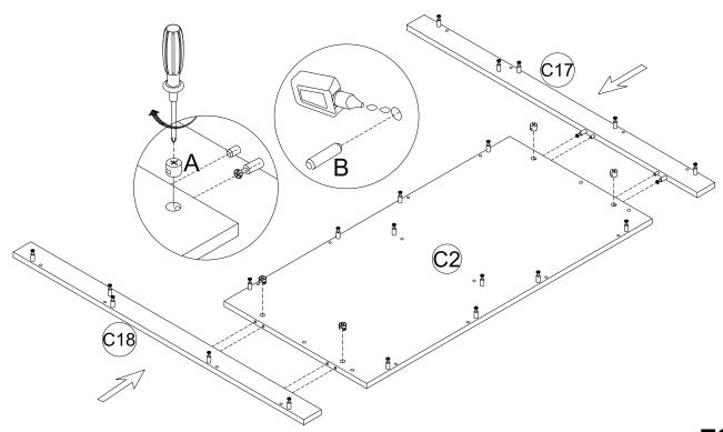
Step 16: Attach Left Front Panel(C17) and Right Front Panel(C18) and Headboard Front Panel(C2) to the Headboard Left Side Panel(C3) and Headboard Right Side Panel(C4) and Shelf Panel(C8/C9). And use a Phillips Head Screw to turn the Cam Lock(A) to lock into the head of the Cam Pin(A).
