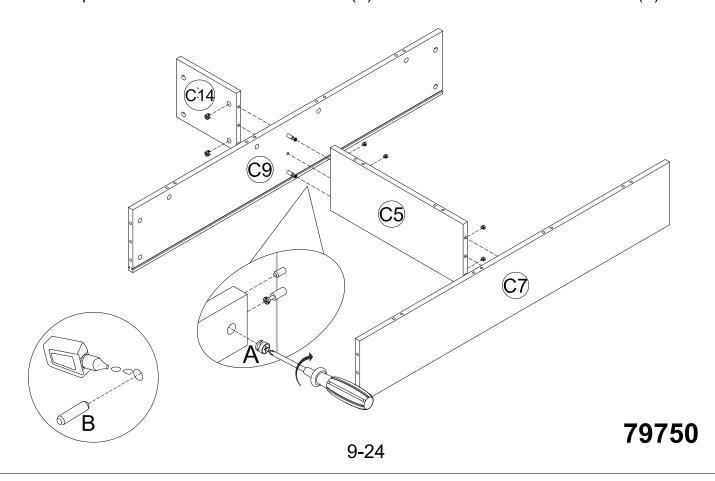
Step 8: Attach Shelf Panel(C8) to the Support Panel(C14). And use a Phillips Head Screw to turn the Cam Lock(A) to lock into the head of the Cam Pin(A).
