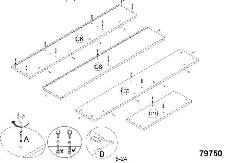
Step 2: Insert the Dowel(B) into the Middle Support Panel(C5) and Shelf Panel(C9)and Support Panel(C11/C12). Use Phillips Head Screw to insert the Cam Pin(A) to the Shelf Panel(C9) and the Front Rail(C1).
