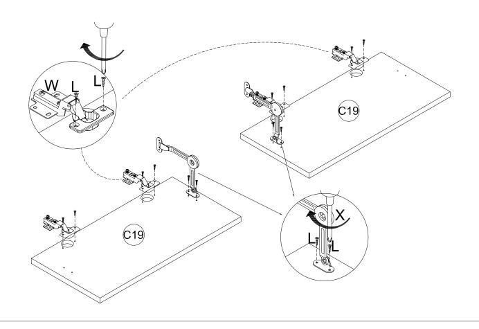
Step 19: Use a Phillips Head Screw Driver to attach hinge (W) to the shelf panel(C9). Adjust and level door panels first before attaching hinge (X). Please see below for adjustment direction.
