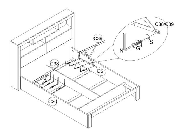
Step 30: Use Hex Key(R) and Wrench(N) to attach Slats(C35) and Gas Lift(C38/C39) with Bolt(K) and Washer(R) and Hexagonal Nuts(J).
